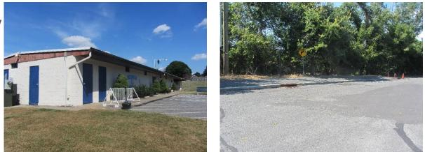
Parking spots along the western side of the lot can be replaced with porous asphalt to capture and infiltrate stormwater. Rain gardens adjacent to the building can capture, treat, and infiltrate roof runoff. A preliminary soil assessment suggests that the soils have suitable drainage characteristics for green infrastructure.
