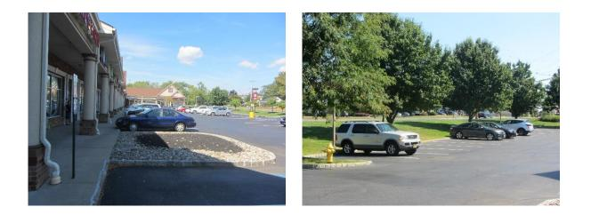
Parking spots in front of the building can be replaced with porous asphalt to capture and infiltrate stormwater runoff. Downspouts from the roof can be disconnected and directed into a rain garden. A preliminary soil assessment suggests that the soils have suitable drainage characteristics for green infrastructure.
