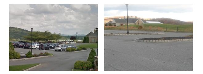
Parking islands can be replaced with tree filter boxes to capture, treat, and infiltrate stormwater runoff and improve the aesthetic of the parking lot. A preliminary soil assessment suggests that the soils have suitable drainage characteristics for green infrastructure.
