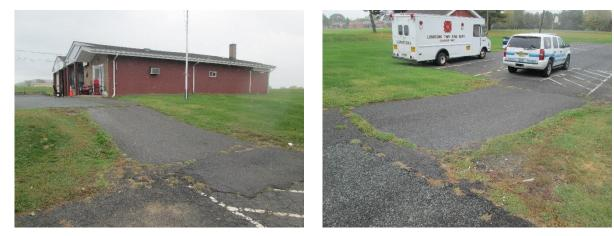
Runoff from the rooftop can be disconnected and drain into a rainwater harvesting system. Installing two rain gardens adjacent to the parking lot can capture, treat, and infiltrate runoff from the parking lots. A preliminary soil assessment suggests that the soils have suitable drainage characteristics for green infrastructure.
