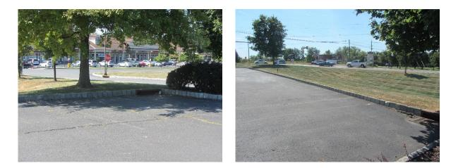
Parking spots can be replaced with porous asphalt to capture and infiltrate stormwater. A preliminary soil assessment suggests that the soils have suitable drainage characteristics for green infrastructure.
